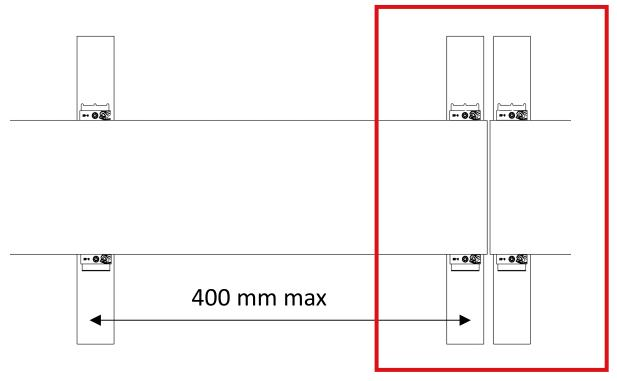
Double joisting at the ends of the boards
